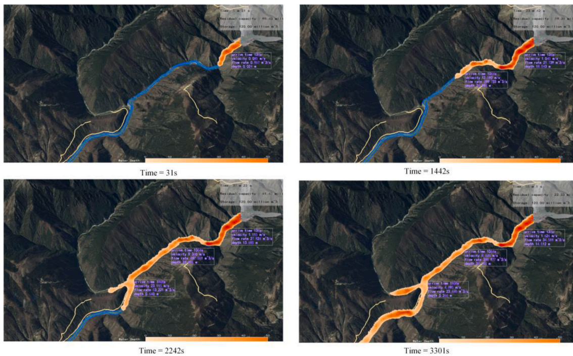
Fig. 12. The spatiotemporal process of a dam-break flood (case 1).
